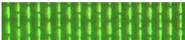
The green output only from an RGB system showing 18 pixels
